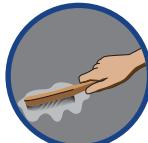
Remove all dirt, loose paint and flakes using wire mesh.
