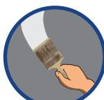
Apply one coat of Seal-O-Prime/BP Cement Primer WT suitably diluted and dry it overnight. Two coats are recommended for better results.
