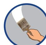
Apply the second coat only when the first coat is dry. Do not overthin. Do not apply when ambient temperature is below 10°C or more than 40°C.
